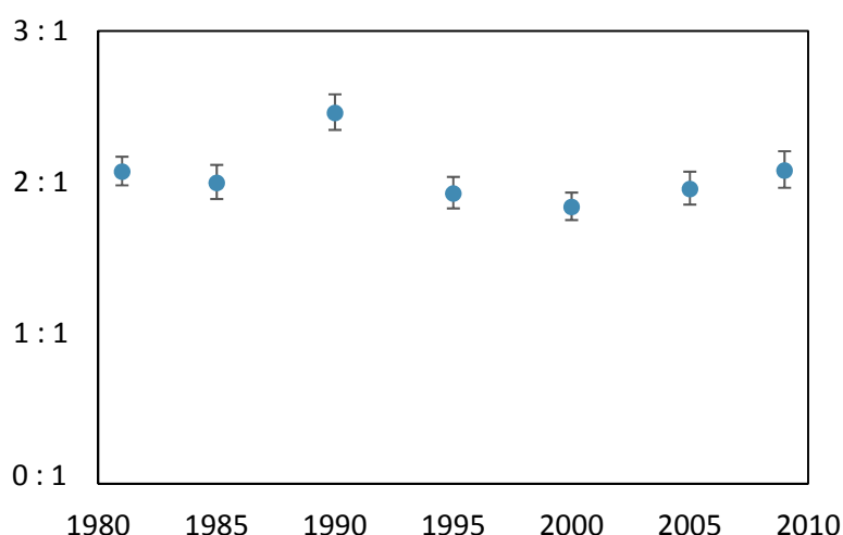
Figure 2. Edible energy efficiency (EEE) for Canada from 1981 to 2009. The vertical bars represent uncertainty in estimates of the energy intensity of fertilizer and pesticides.
